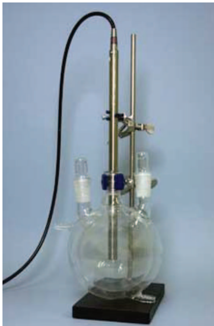
Figure 5. The RamanFlex offers a simple and convenient way to monitor reactions
